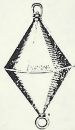
JA 252. — Conical Shape Mooring Buoy. 20-gauge galvanised iron. 3/4 in. galvanised rod. Buoy revolves round rod. Eye at top, swivel below. Size 5ft. x 2ft. 6in., £4/10/-; 3ft. x 2ft., £3 each
