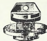
JA 119.—Brass Boat Plug. Screw type. A slot in screw of plug enables boat to drain without unscrewing plug right out. Sizes, each— In. 1/2 3/4 1 Price 4/6 5/6 6/6 6/9
